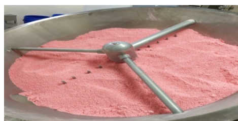
Figure.7 Granules being dried in FBD 150 Kg (improvement) Source: Processed Data (2021)
