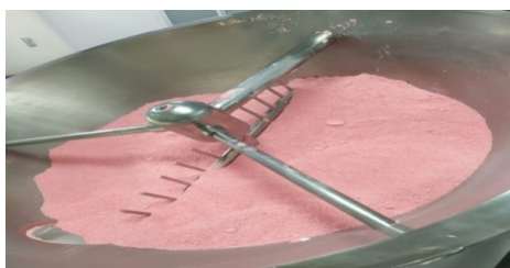
Figure 5 Granules being dried in FBD 150 Kg (before improvement) Source: Processed Data (2021)
