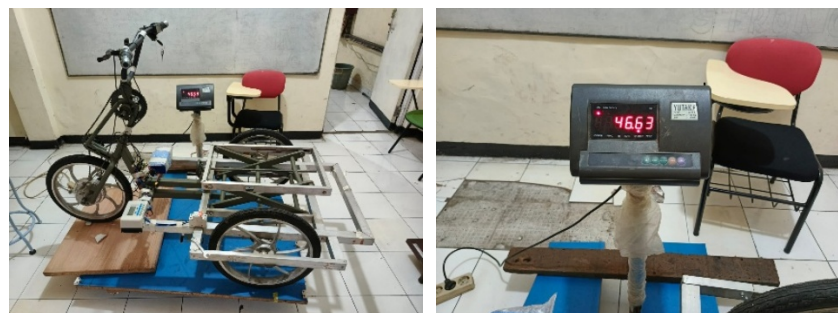
Figure 14. Weighing the handcycle frame
