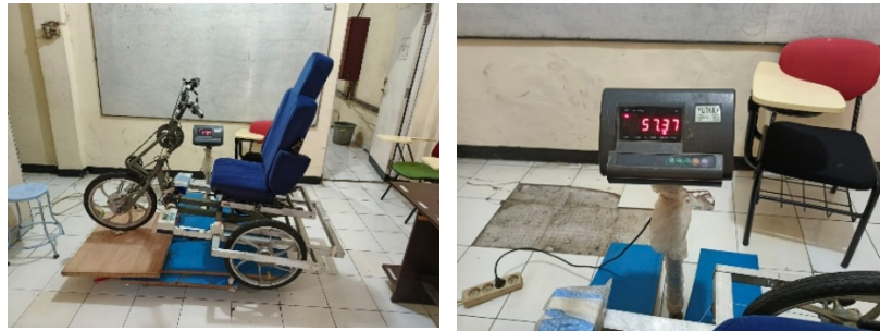
Figure 15. Weighing the handcycle frame and seat
