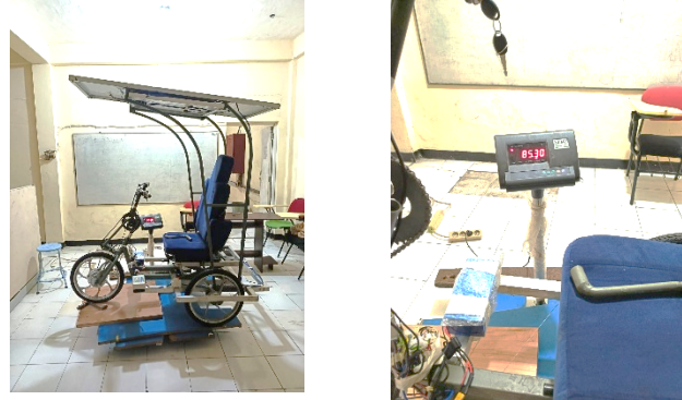
Figure 16. Weighing the handcycle frame, seat and panel
