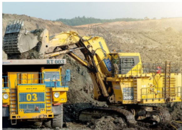
Figure 3. Electrification Unit (PC3000E & HD BELAZ) of PT Bukit Asam Tbk
