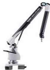
Figure 3. CMM Tipe Potable Source : Hexagon Manufacturing Intelligence
