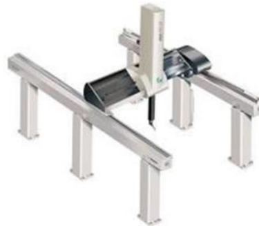
Figure 2. CMM Gantry Type Source: Hexagon Manufacturing Intelligence
