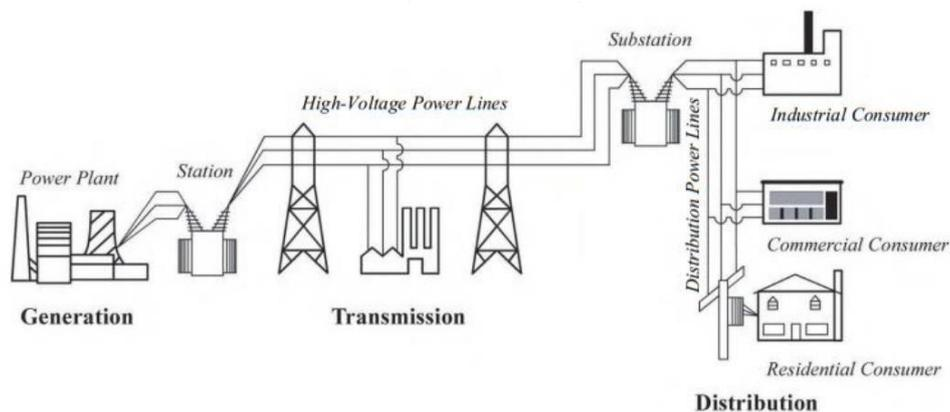
Figure 1. Electricity System: Generation, Transmission and Distribution
