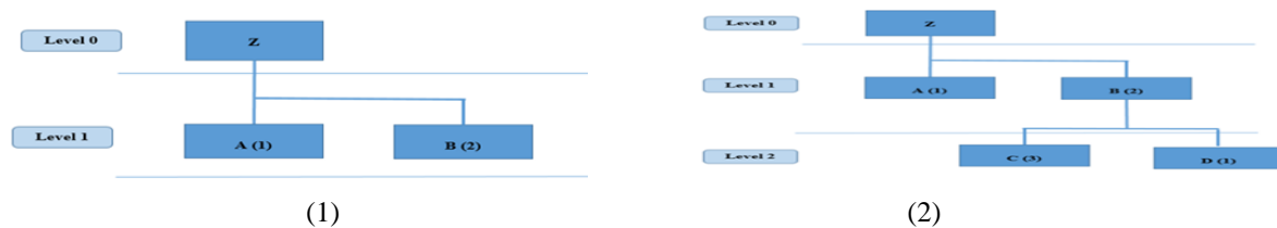
Picture 3. Single Level Product Structure (1) and Multi Level Structure (2)
